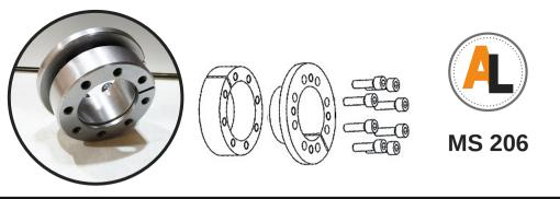
**MS 206** – This is suitable for medium to high torques. Since the mounting is small, the installation time is also reduced. It is also economically advantageous. Any application which requires an accurate axial positioning, this Locking assembly cannot be used. This design has a single taper.
